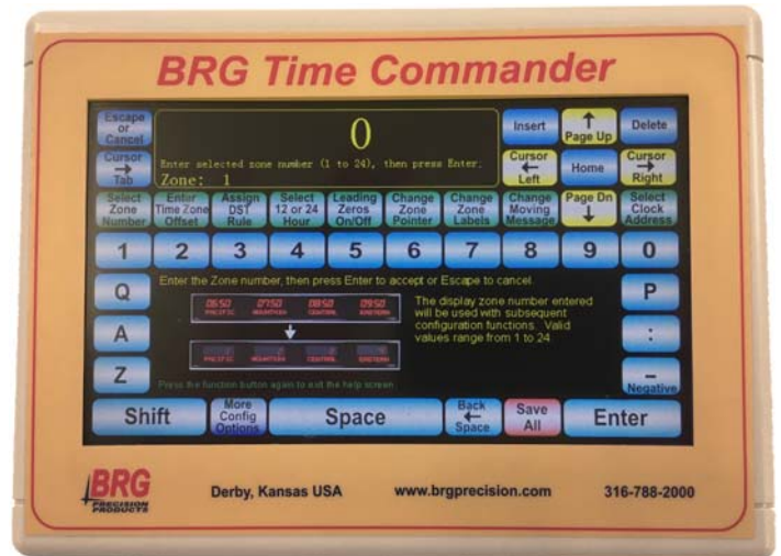
Above: Showing the programming of a 6610H 4 Zone Time Zone Clock
