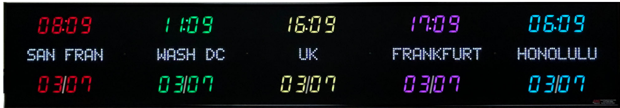
Model 6613D - 1.8" bar segment time & date, 1.2" zone labels, 5 zones
