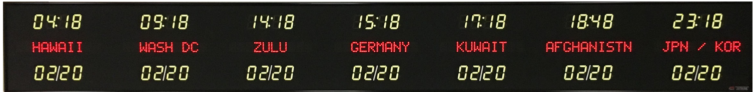
Model 6613N - 1.8" bar segment time & date, 1.2" zone labels, 7 zones
