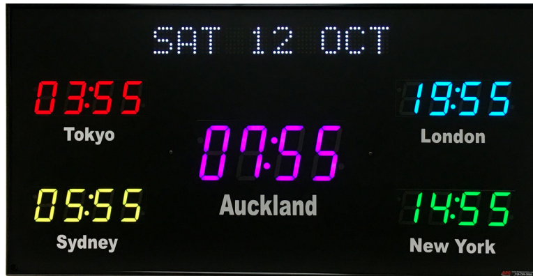
Model 664E - 4.0" center zone time & 1.5" vinyl zone labels, 2.5" perimeter zones time & 1.0" vinyl zone labels, 2.0" 10 character date, 5 zones
