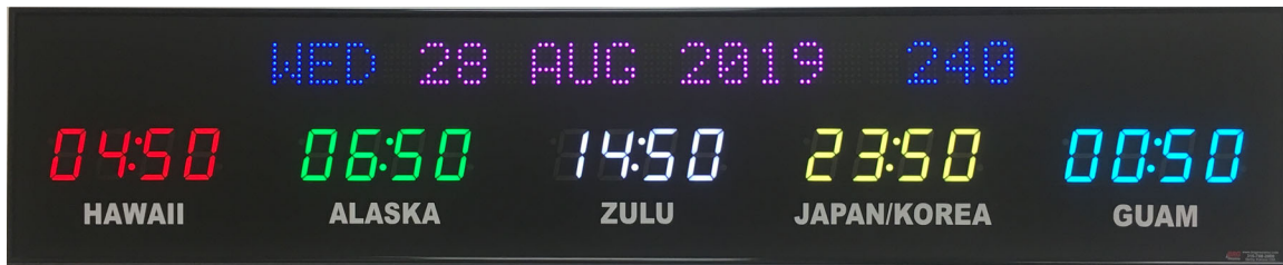
Model 668L - 2.5" time, 2.0" - 20 digit date, 1.0" zone labels, 5 zones
