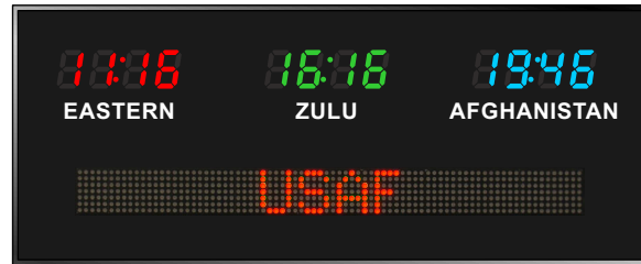
Model 669B - 1.8" time, 0.75" white vinyl zone labels, 2.0" dot matrix message display 24" wide, 3 zones
